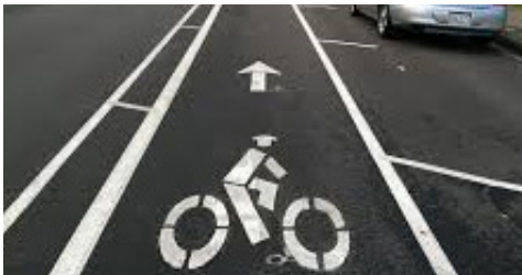
Example of Buffered Bike Lanes - Source: Kimley-Horn
