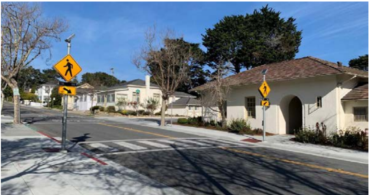
Rectangular Rapid Flashing Beacon Outside Monterey City Hall - Source: City of Monterey
